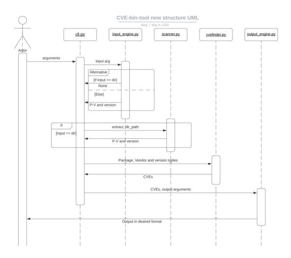
Above, UML diagram explains general flow from user calling *cli.py* with arguments to *output\_engine* displaying output to the user.
